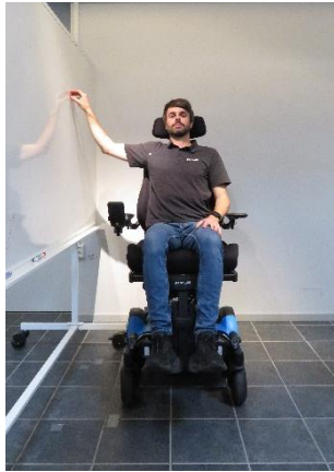
Figure 8: Measurement of shoulder abduction, elevation 8" (20 cm) (this was the maximum seat height in the study of Sabari et al. 2016), at 14" (35.56 cm) distance from the wall.
