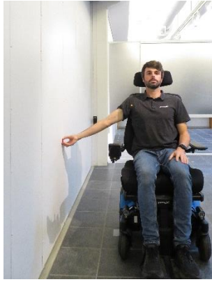
Figure 13: Measurement of maximum possible reach height for a minimum seat height 17.5" (44.45 cm), at 19" (48 cm) distance from the wall. The tests were performed with a shoulder abduction of 60°
