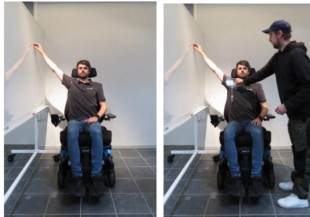
Figure 7: Measurement of shoulder abduction, minimum seat height of 17.5" (44.45 cm) from the floor, at 14" (35.56 cm) distance from the wall.
