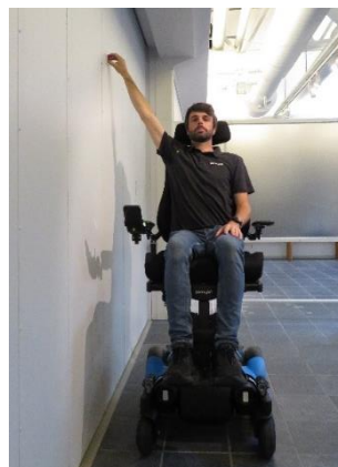
Figure 6: Power wheelchair positioned 9.45" (24 cm) from the wall with participant in maximum shoulder abduction while positioned in a 12" (30.5 cm) elevated seat.
