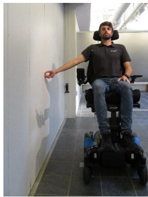
Figure 15: Measurement of maximum possible reach height for a maximum seat height 29.8" (75.7 cm), 19" (48 cm) distance from the wall. The tests were performed with a shoulder abduction of 60°
