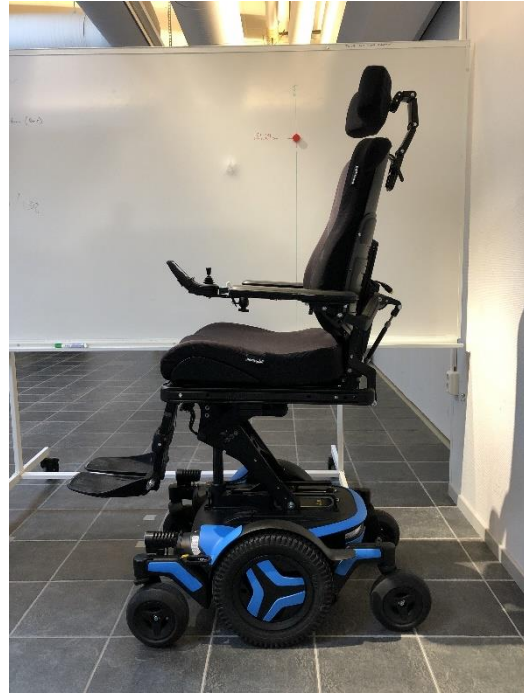
Figure 2: Maximum seat to floor height of 29.8" or 75.7 cm (30.5 cm of seat elevation)
