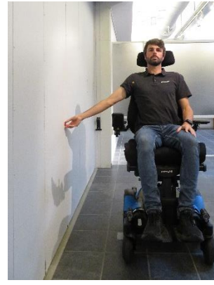
Figure 14: Measurement of maximum possible reach height for a seat height 25.5" (64.45 cm), at 19" (48 cm) distance from the wall. Test were performed with a shoulder abduction of 60°
