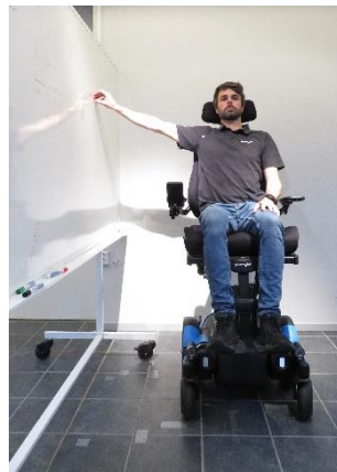
Figure 12: Measurement of shoulder abduction, maximum elevation 12" (30.5 cm), at 20" (50 cm) distance from the wall.
