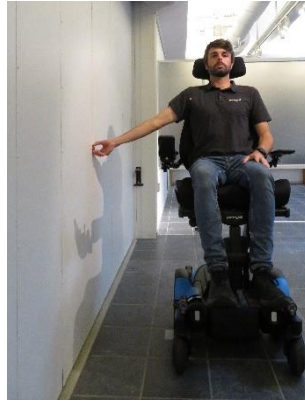
Figure 5: Positioning to measure the maximum height on the wall that could be reached by the test person, with 60° range of motion of the shoulder.
