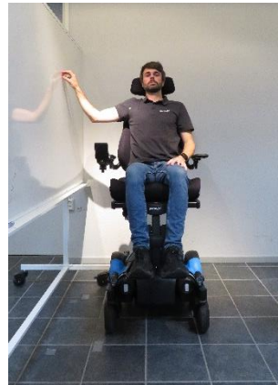
Figure 11: Measurement of shoulder abduction, maximum elevation 12" (30.5 cm), at 14" (35.56 cm) distance from the wall.
