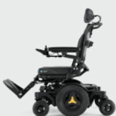
Power leg rest 80°–140° (>480 mm seat depth) 90°–150° (≤480 mm seat depth) Manual leg rest 80°–135°
