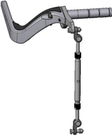
Armrest kit “narrow” Armrest adjustable 380 – 480 mm
