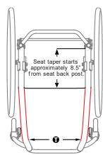
**FOOTEST WIDTH** I or V Select either a Standard Front End I if no Seat Taper T is selected or a V-Front End V if a Seat Taper T is selected.
